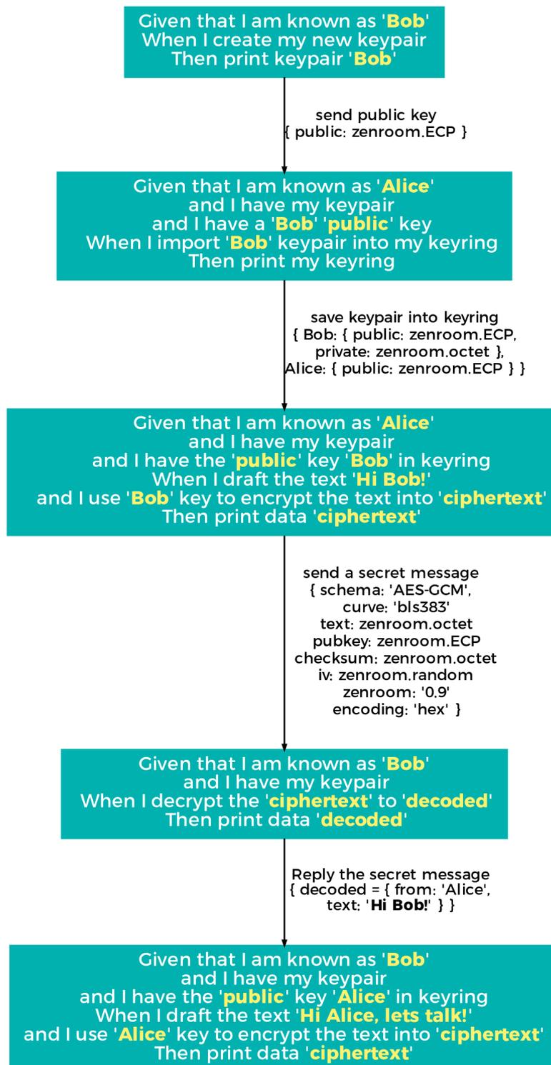
This simplified flow diagram shows **actual Zencode** that can be executed, highlighting variables that are normally just surrounded by single quotes. Between each code block, which is executed asynchronously as required and at different times, there is a schema which indicates the shape of data in output.
