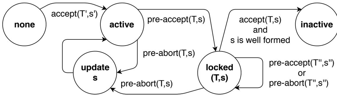
Figure 6: State machine representing a the life cycle of Chainspace objects.
