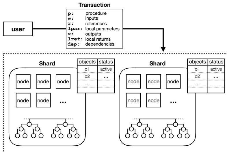
Figure 3: Design overview of Chainspace system, showing the interaction between users, transactions, objects and nodes in shards.
