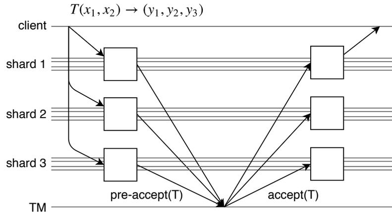
Figure 5: An example execution of L-SBAC for a valid transaction  $T(x_1, x_2) \rightarrow (y_1, y_2, y_3)$  with two inputs ( $x_1$  and  $x_2$ , both are active) and three outputs ( $y_1, y_2, y_3$ ), where the final decision is `accept(T)`.
