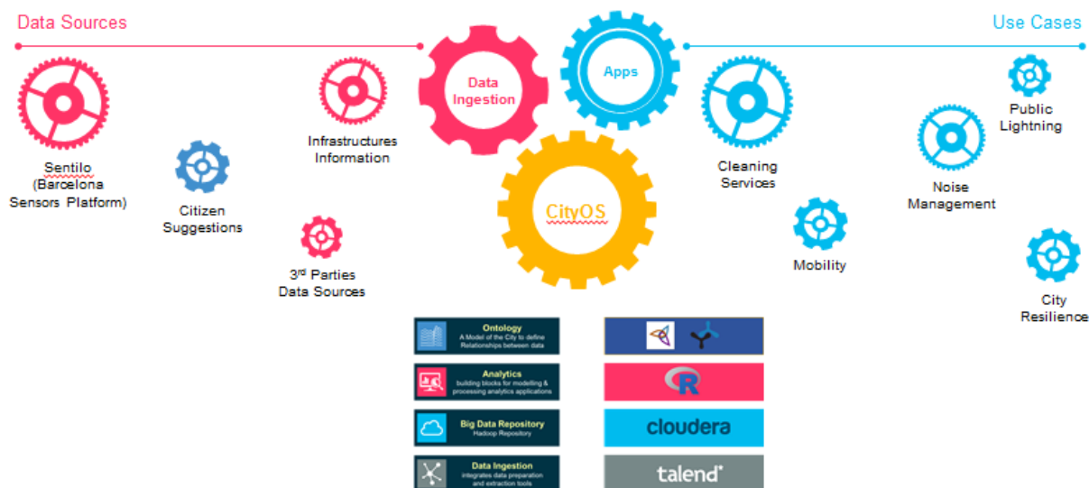
Figure 3: CityOS, a graphical overview of its functions.
